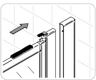
8 Insert the door into the wall compensator.
