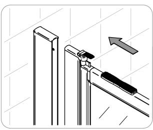
Insert the door into the wall compensator.
