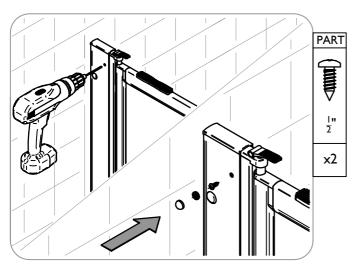
25 Drill (using a 3.5mm bit) and screw lockup holes (x2) in door compensator.
