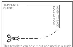
This template can be cut out and used as a guide to trim the fixed panel coving foot.
