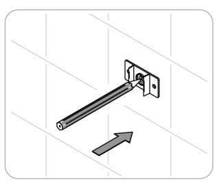
Unclip the marking plate and align with the previously marked points. Mark the centre hole for drilling. **DO NOT DRILL OUTER POINTS**
