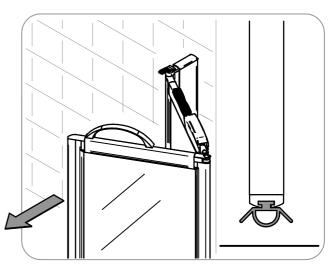
Test the door operation to ensure the doors meet and the floor seal does not drag.
