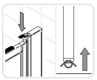
**77** Press the release lever to raise the door.
